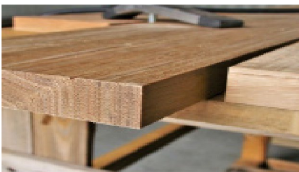
Clean corner on exit side with no "blowout".
