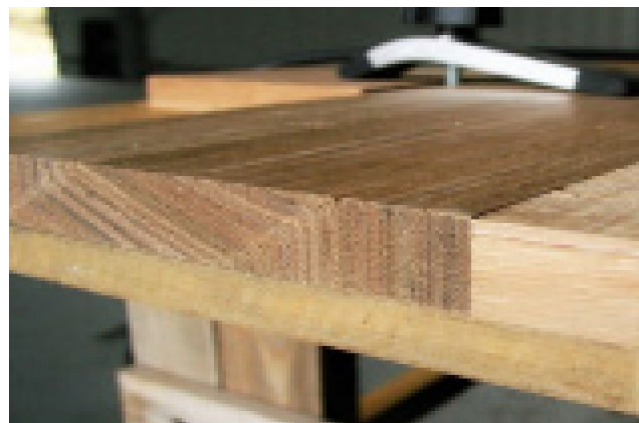
End Grain Routing with support piece.
