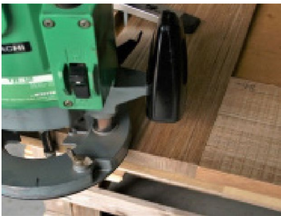
Clean corner on exit side with no "blowout".
